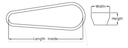
$\begin{array}{ll} \text{Datum Llength} = 3150 \\ \text{Height} & = 10 \\ \text{Length inside} & = 3100 \\ \text{Width} & = 17 \end{array}$
